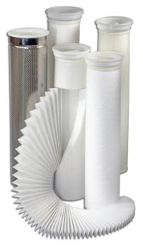
A fully homogeneous welded filter element in one material (Polypropylene or Polyester) with integrated gasket function and length compensation for accurately fitting in the restrainer basket.
