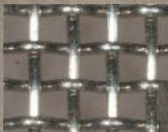
stainless steel mesh 250µm magnified plain weave
